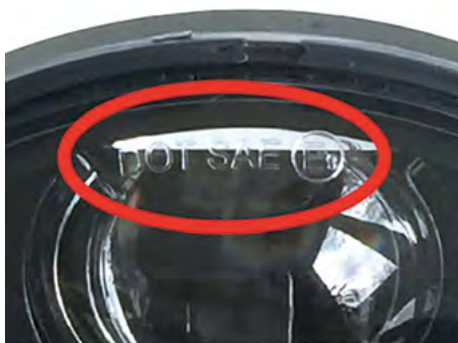
Picture shows a forgery of the ECE homologation markings
