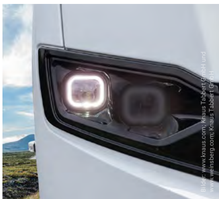
Illustration shows a simulation of a defective light guide
